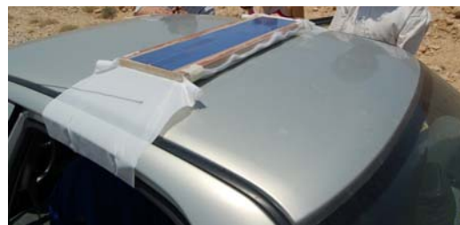
Figure 40: Solar Array Wind Cooling Test.
