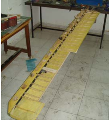
Figure 38: Wing Bending NDT
